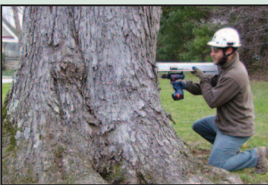
Tadd Leyman, ISA Certified Arborist, uses our Resistograph on a maple tree in Villanova.
