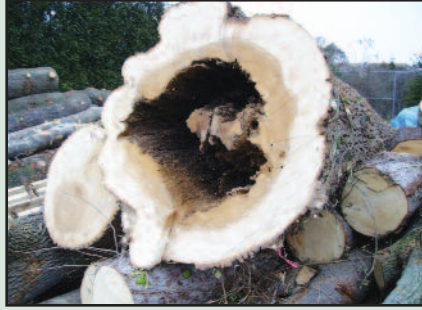
This large ash tree appeared to have a solid trunk. We used our resistograph machine to test the trunk and found the tree to be hollow.
